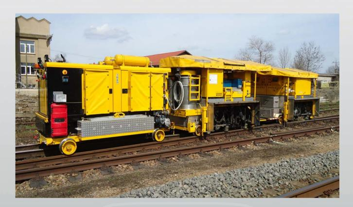
The LRGM 2-12 is a turnout grinding machine for the machining of the rail head. The machine composes two coupled grinding units LRGM 1-6, each with 6 grinding spindles with independent angular adjustment. They are driven by 7,5 kW to 15 kW frequency controlled electrical motors. The grinding process is monitored automatically. The machine can be equipped with an integrated laser measurement system for the analysis of the transverse and longitudinal rail head profile.
