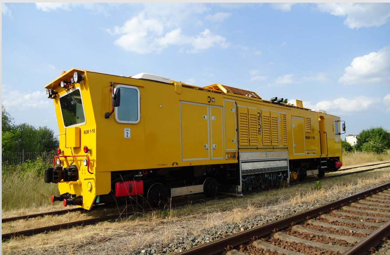
The rail grinder RGM 1-10 is a rail-borne machine which has 10 grinding spindles with independent angular adjustment. Each of the spindles is driven by a frequency-controlled electrical motor. The computer monitored grinding process is controlled with touch pad by the operator inside of the cabin.
