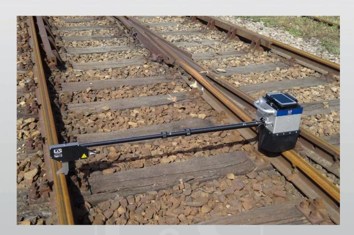
The TMD 1-2 is an efficient solution for the detection of transverse profile on all rails. The measuring device TMD 1-2 is applicable for grooved rails and standard Vignol rails.
